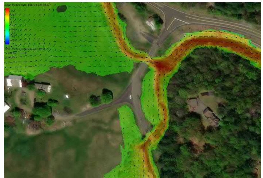
Figure:11 SRH-2D Hydrodynamic Modeling Results: 50-Year Riverine Flood, Proposed Condition
