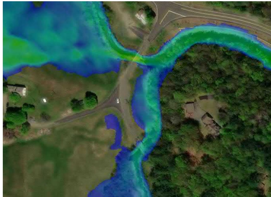
Figure:10 SRH-2D Hydrodynamic Modeling Results: 25-Year Riverine Flood, Proposed Condition
