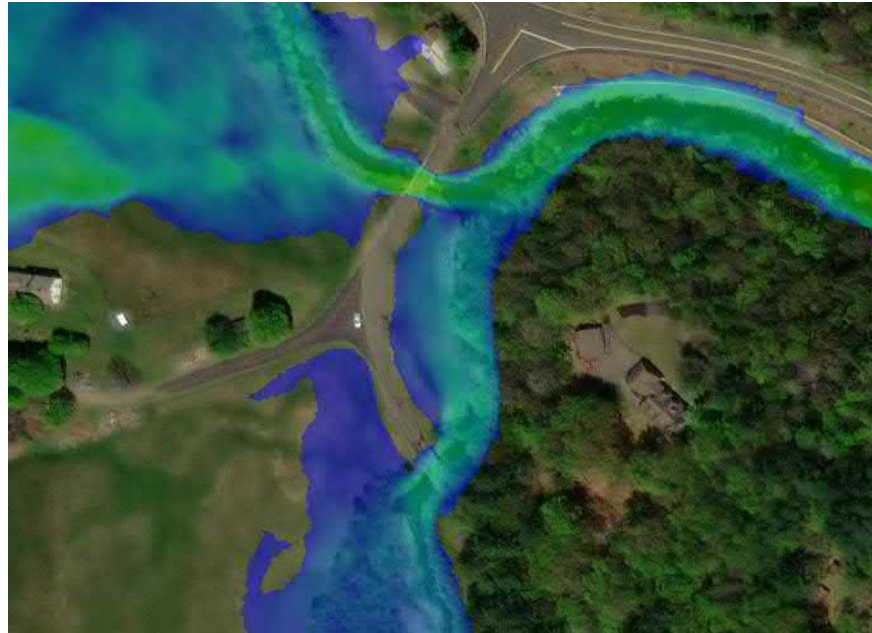
Figure:12 SRH-2D Hydrodynamic Modeling Results: 100-Year Riverine Flood, Proposed Condition
