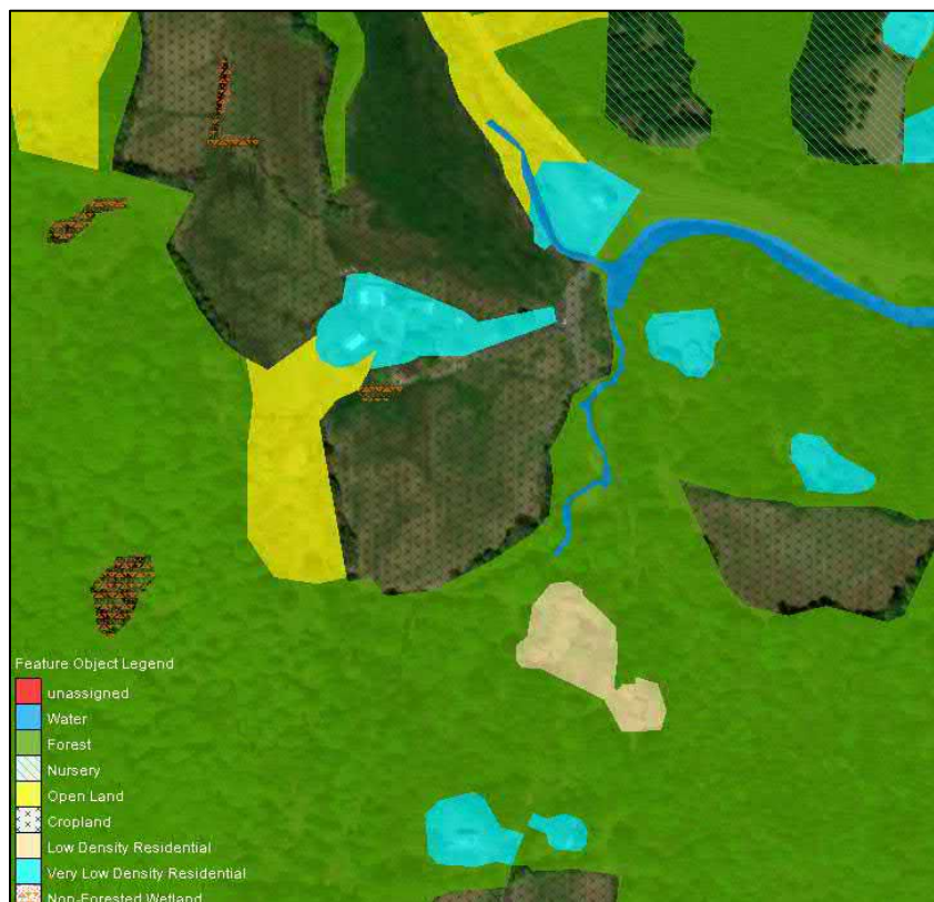
Figure 4-4 Land Use Coverage used in SRH-2D Model
