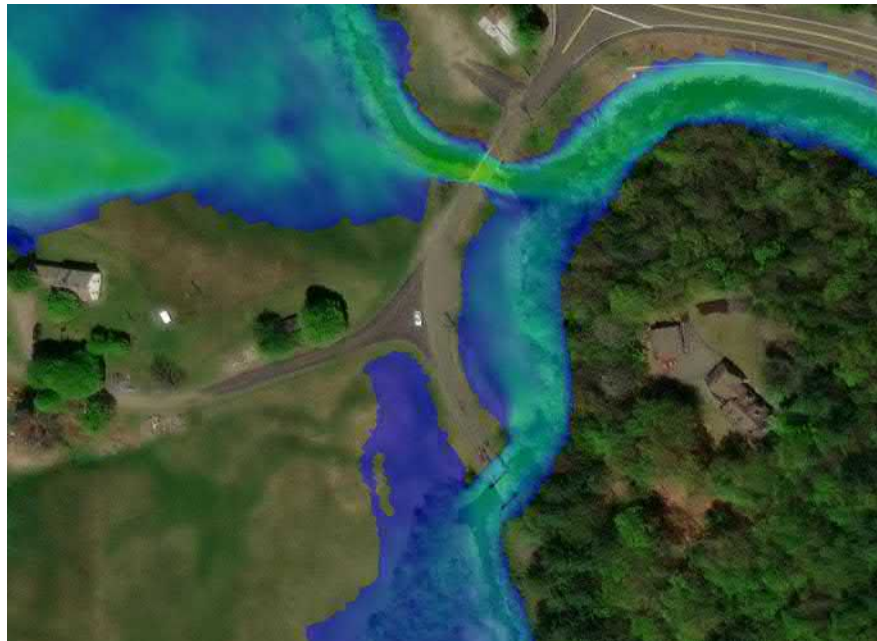
Figure:7 SRH-2D Hydrodynamic Modeling Results: 50-Year Riverine Flood, Existing Condition
