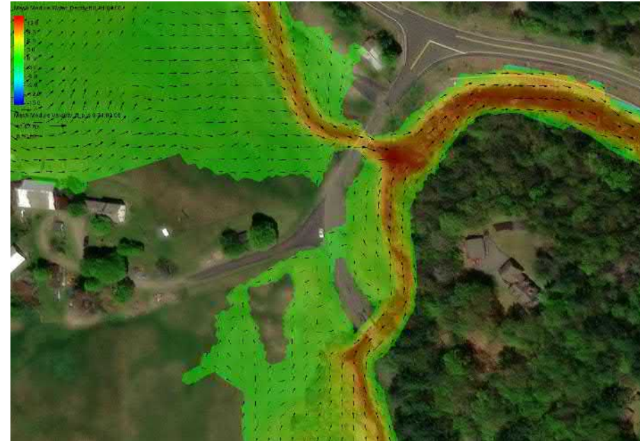
Figure:8 SRH-2D Hydrodynamic Modeling Results: 100-Year Riverine Flood, Existing Condition
