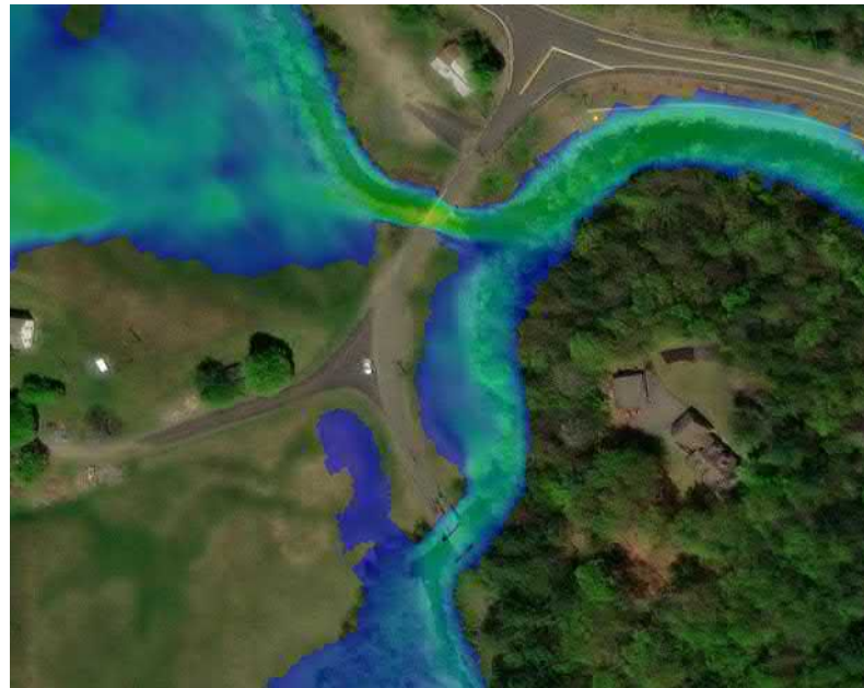
Figure:6 SRH-2D Hydrodynamic Modeling Results: 25-Year Riverine Flood, Existing Condition
