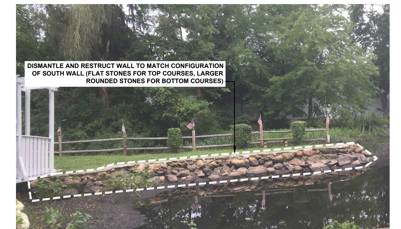
11 LAGOON WALL RECONSTRUCTION NOT TO SCALE
