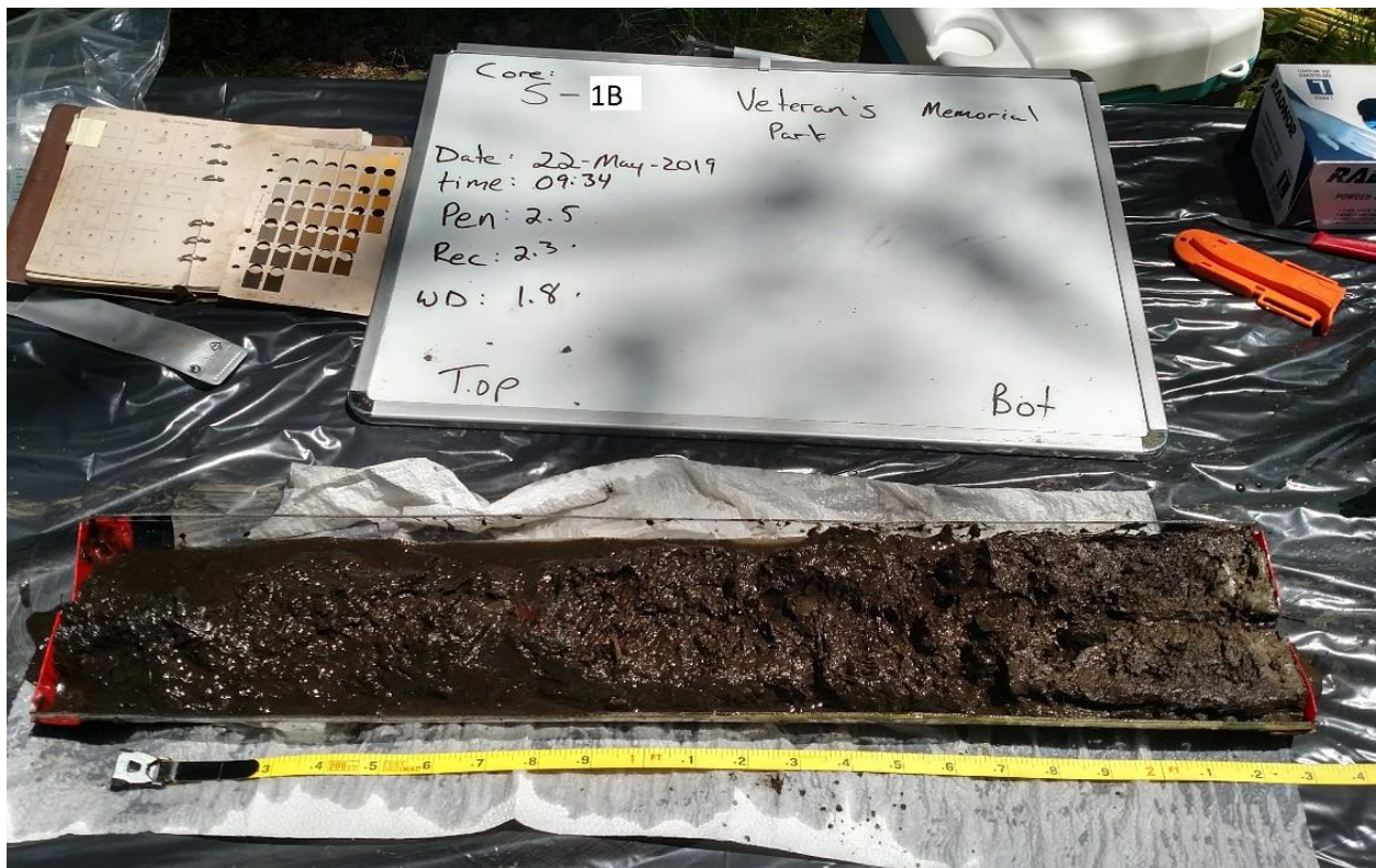
Sediment Core from Location S-1B (surface to depth from left to right)
