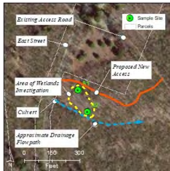
Figure 8. Area of wetland investigation showing the location of the drainage flow path and proposed new access. The sample sites correspond to the wetland delineation forms in Appendix D.
