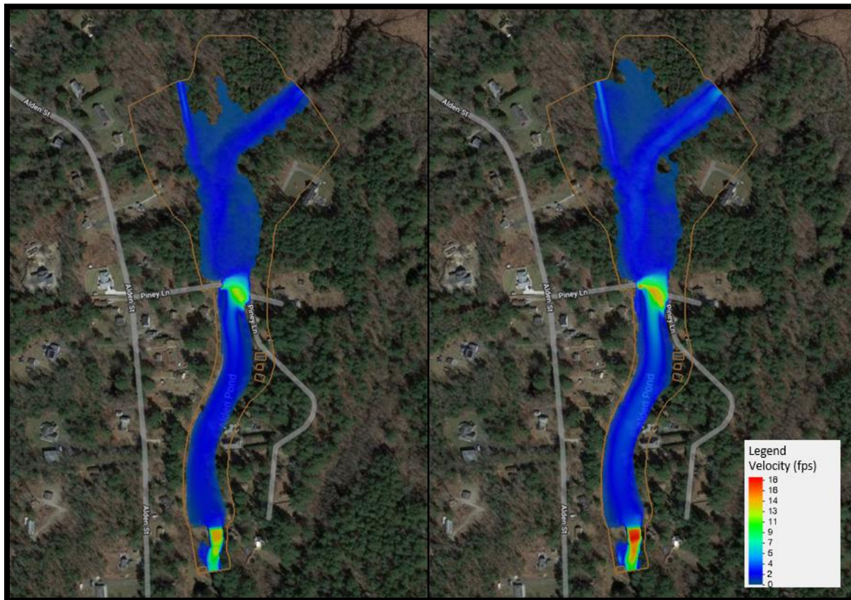
Figure 5-5. Existing Velocity Magnitude – Entire Reach
