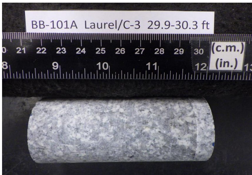
After cutting and grinding
